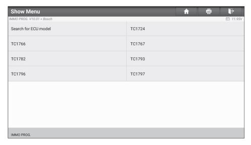
d. Check ECU model (printed on the sticker on the back of your Engine), enter the engine type in the dialogue box (Take the following picture as an example, the engine type should be MED17.7.7).
